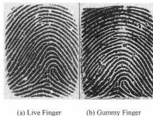
Figure 4.3 The sample images of fingers which derive from the same finger and were displayed on the screen when being scanned by the capacitive sensor of Device H.
